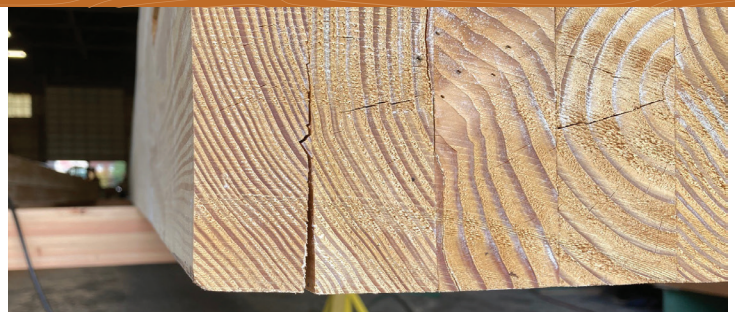
Douglas fir glulam treated with waterborne preservatives
